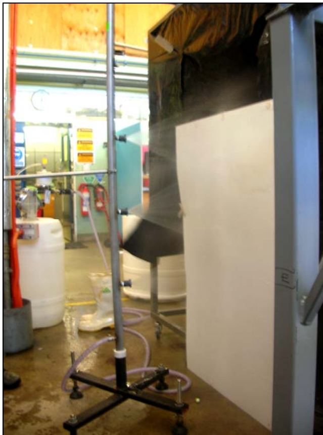
Figure 1. A photograph of a spray applicator used in the study to deliver water or Inspexx 200 rinse to inoculated meat samples.
