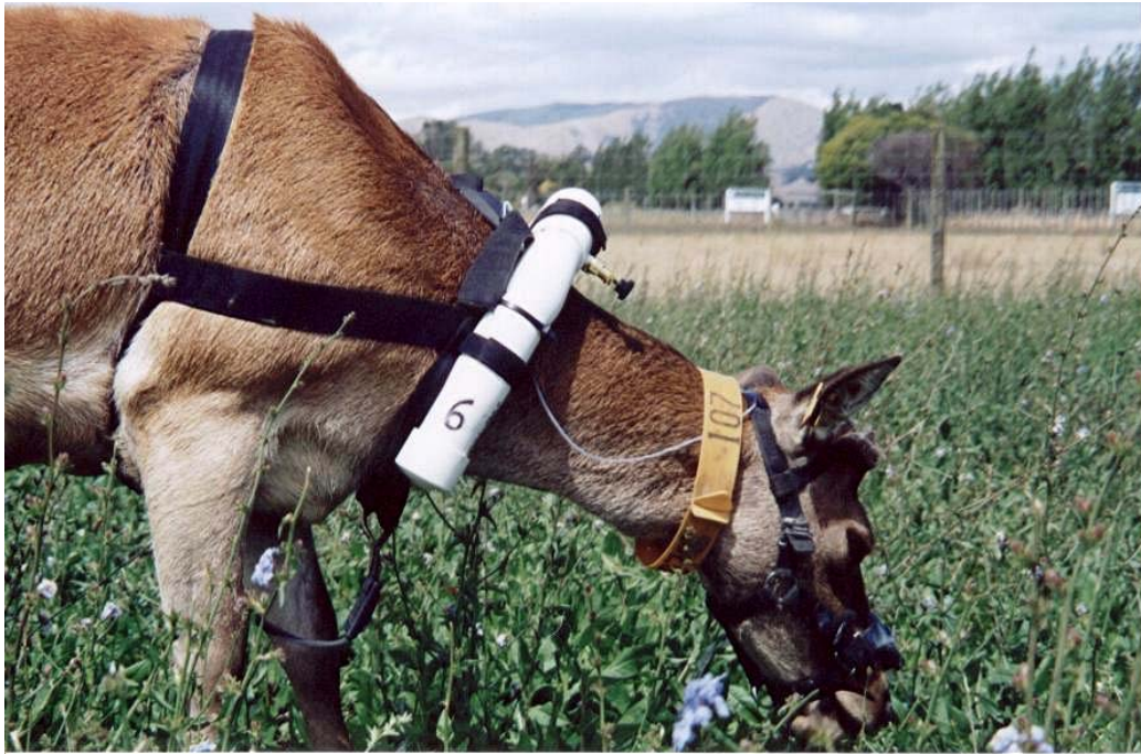
Figure 1. Red deer equipped with methane collection gear, grazing chicory in early March.
