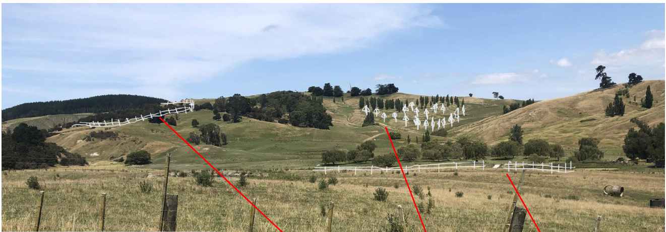
Planned erosion control and waterway actions are sketched onto a photo
